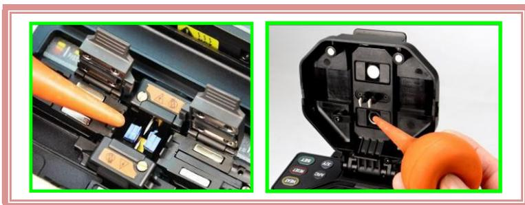
The mirror and objective lens are dusty after a long time without routine maintenance, resulting in whitening and fuzzy black-clad of fiber image.
