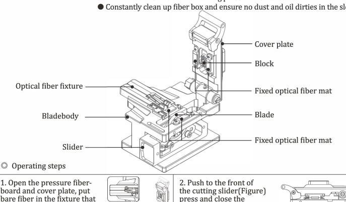
1. Open the pressure fiberboard and cover plate, put bare fiber in the fixture that was stripped coating (125mm/900mm) according to user's requirement to ensure cutting length.
