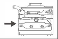
5. Open cover plate and pressure fiberboard, then take out the fiber. In order to avoid damaging the fiber, fiber face don't touch anything after take it out.
